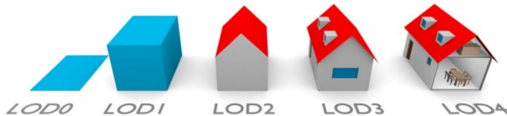
Fig. 1. The five LODs of CityGML 2.0. The geometric detail and the semantic complexity increase, ending with the LOD4 containing indoor features
